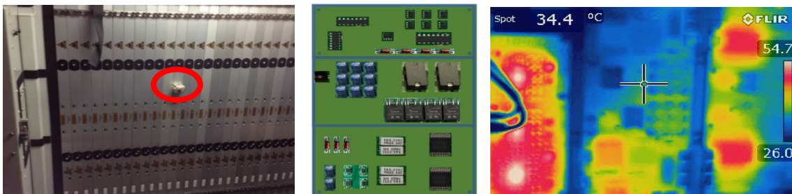
Figure 5: a) Stacking of PCBs in radar with installed vibration sensor (red circle); b) Typical layout of printed circuit board; c) Thermal camera image of temperature distribution.
