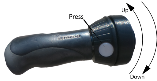
Figure 4: The final prototype of Brotate and its supported actions.
