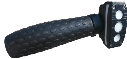
Figure 5: The final version of Tribike with three action buttons. The device uses the same button patterns as standard mobile phone in-line remotes.
