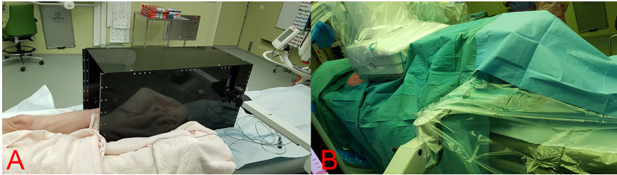
Online Figure 1: A: An in-house designed box, made of black non-transparent Perspex, enveloping the foot to shield the LSCI laser from its surroundings. B: Box covered with sterile sheets during the procedure.
