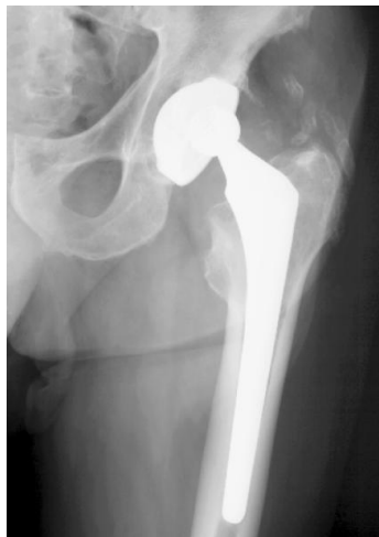
Figure 2.2. An example of liner wear causing eccentric seating of the head, adapted from [1]
