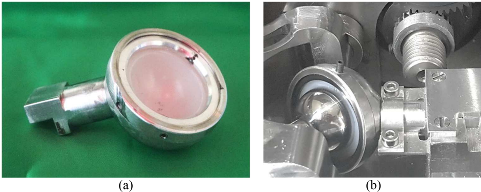
Figure 5.9. (a) Liner inside of cup and (b) positions of head and liner in the hip simulator
