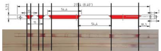
Figure 3: Pressure distribution of a wedge-lock retainer visualized by a pressure sensitive foil.
