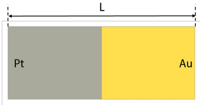
Figure 3.1: Schematics showing the fabricated (b) Pt-Au bimetallic electrode for flow characterization experiments, having a total length L = 10 mm.
