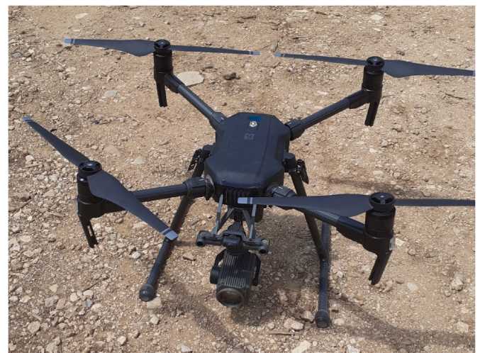
Fig. 2. Unmanned Aerial Vehicle (UAV) system, M210 V2 quad copter with a Zen muse digital camera onboard. The UAV camera acquire images on the blue, green, red bands at high spatial resolution (10 cm) at 70 m flight height. (For interpretation of the references to colour in this figure legend, the reader is referred to the Web version of this article.)
