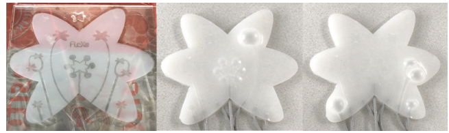
Figure 3: Flexo Atom co-designed to be like abstract hands with 9 inflatable finger like pockets.
