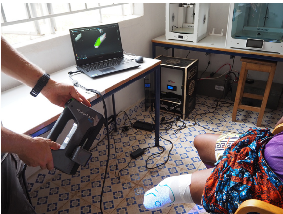
Fig. 1. Scanning of the stump with the Ein-scanner Pro Plus.
