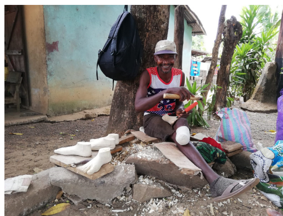
Fig. 7. The prosthetic foot is made from wood, in the size of the person's foot, produced by a local hospital patient who is specialized in wood carving.
