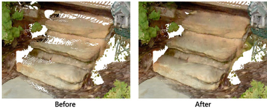
Fig. 3.14 Inpainting a 3D point cloud separately for geometry and colors and then combining the results. (Reproduced from Väänänen and Lehtola 2019)
