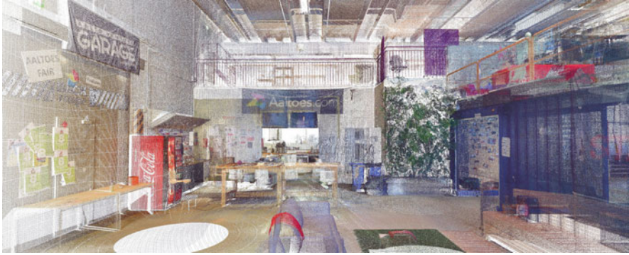
Fig. 3.1 Point cloud of Startup Sauna entrance at Aalto University. (Reproduced from Lehtola et al. 2017)
