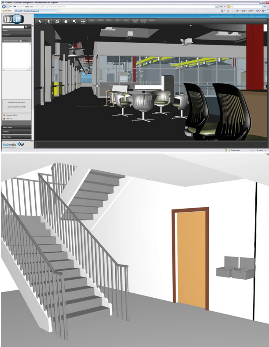
Fig. 3.15 3D BIM models for industry applications, e.g. facility and asset management (top, courtesy of Engworks) and construction (bottom, courtesy of Youbim, youbim.com). Building information modeling (BIM) is important also for various other planning applications
