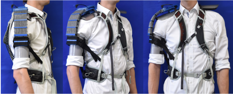
Figure 5.9: Wearable proof-of-concept prototype worn by a healthy subject. This figure illustrates the actuator's potential to achieve close alignment to the body and an overall small size of the resulting assistive device.
