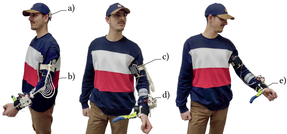
Figure 4.1: The SoftPro Wearable System, worn by a healthy subject. a) e-Cap, b) Assistive Elbow Orthosis, c) CUFF, d) common power supply and control unit, e) Robotic Sixth Finger
