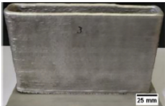
Fig. 32. Rectangular-shaped specimen: 170 mm long, 30 mm width and 120 mm height, and 5 mm radius for the corners [316].
