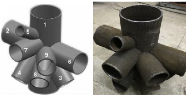
Fig. 60. Case 8 Pipe joint [247]
