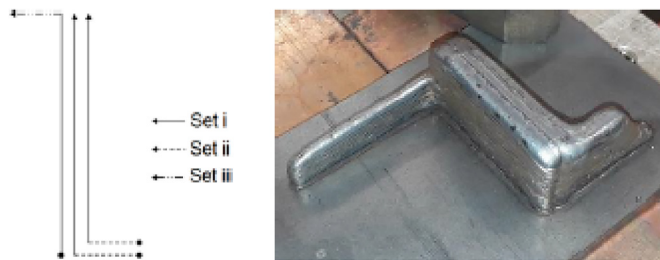
Fig. 31. The top view of the L-shaped path strategy with various wall thicknesses; set i: WFS= 5 m/min and TS=10 mm/s, two tracks (12 mm); set ii: WFS= 2.5 m/min and TS=10 mm/s, two tracks (8 mm), and set #iii: WFS= 1.5 m/min and TS=4 mm/s, single track (4 mm) [269].
