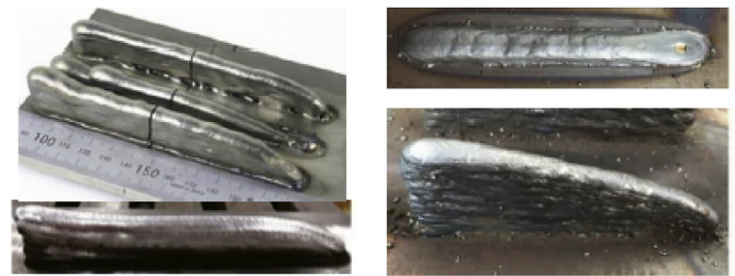
Fig. 15. An irregular appearance of the deposited bead [74,263] (left), single weld bead (right-up), and thin-walled part with 16 layers single-pass [265] (right-bottom).
