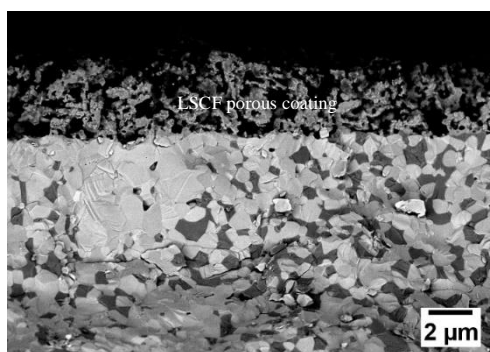
Figure 7.9 Cross section of the coated CF-D.
