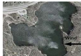
Figure 2. Wind shielding on Holland Lake, illustrated by reflection of visible light on waves (Markfort et al., 2010)
