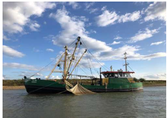
Figure 1. Vessel equipped with a stow net attached to an anchor used for macro- and mesoplastic sampling in the current study.
