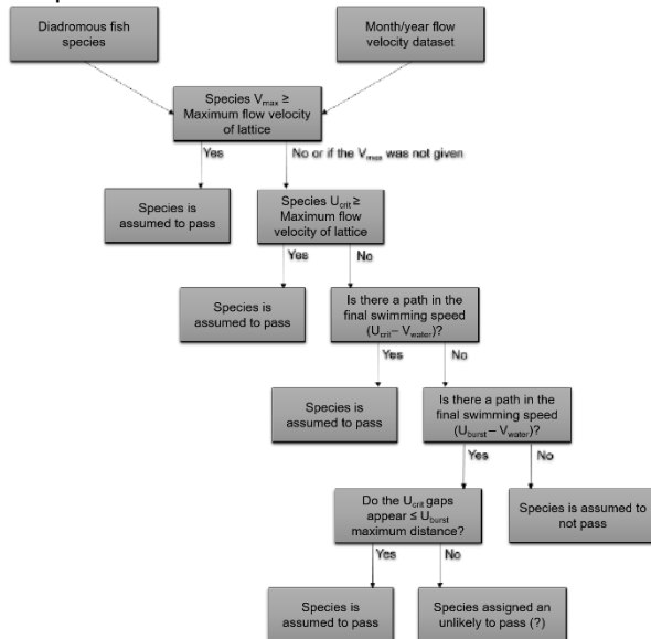
Figure 1. Decision tree for the passability analysis by diadromous fish species of the shore channel inflows.
