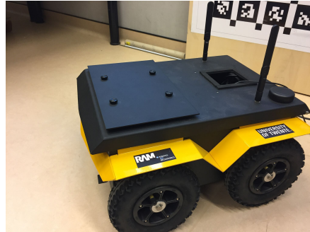
Figure 7: Clearpath Jackal differential drive mobile robot used in the real-world experiments at University of Twente.
