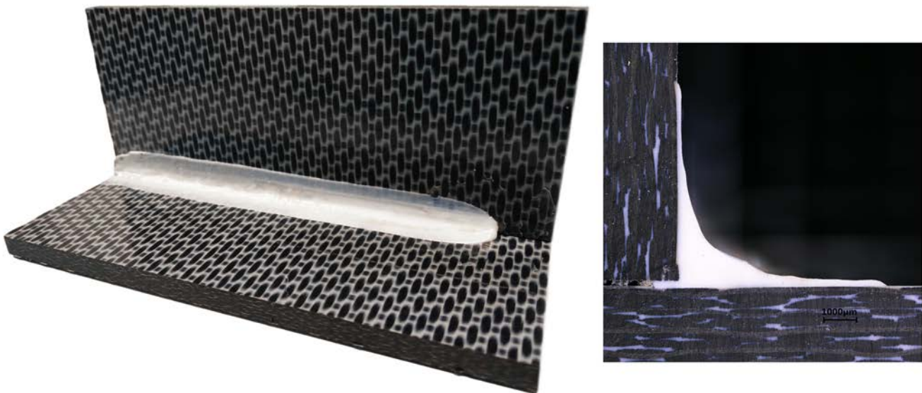
Figure 29: Sample welded with T-CAT REV3. Filler radius of 3 millimeter.
