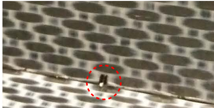
Figure 55: Thermocouple placement in a gap under the stiffener laminate.
