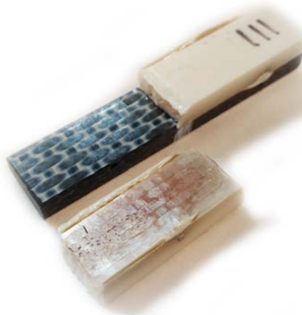
Figure 63: The browning of PPS in sample 111.
