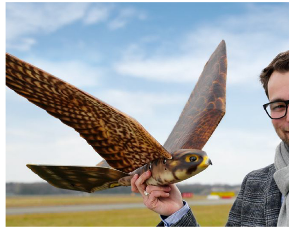
Fig. 10. Robird by Clear Flight Solutions: an artificial falcon to chase birds away from airports.
