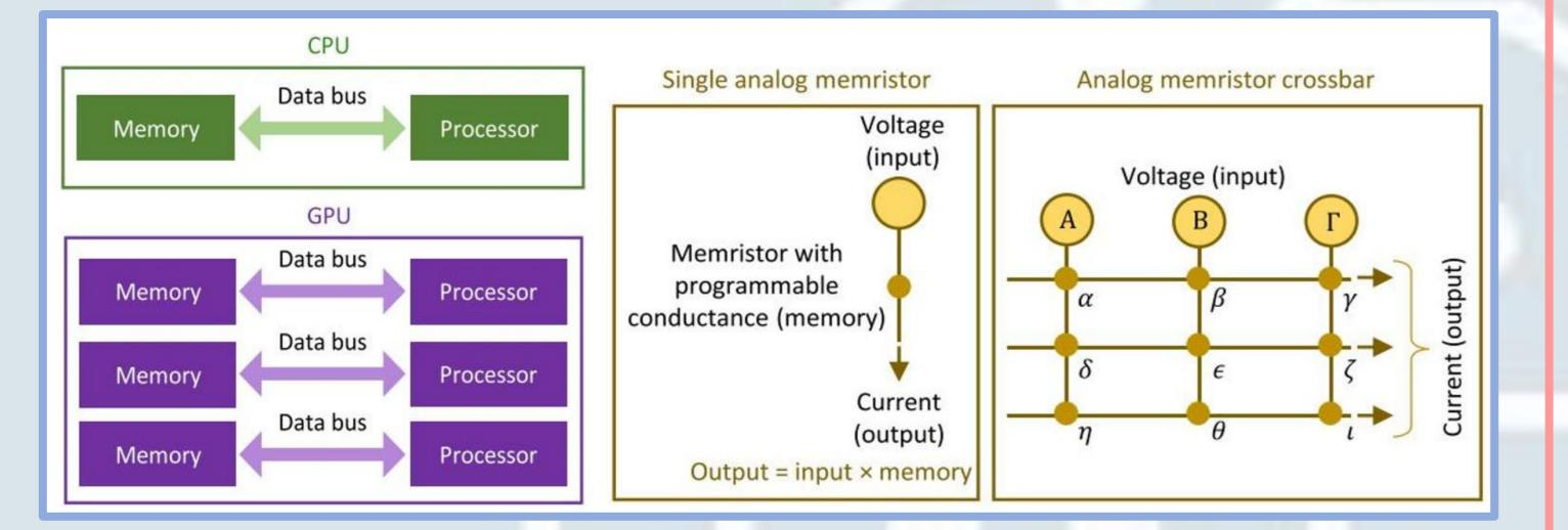
Fig. 1 The computing process in CPU, GPU and memristors.<sup>2</sup>
