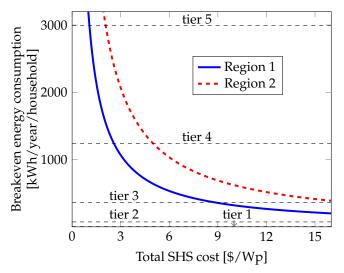
**Figure 4.** Illustrative breakeven annual consumption as a function of SHS upfront costs for two different regions (adapted from [25]). The different tier consumptions of the MTF are also marked for reference. Tier 1 is not clearly visible given the scale of the *y*-axis, as the annual energy consumption for tier 1 level is merely 4.38 kWh.
