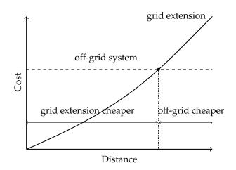
**Figure 3.** Conceptual comparison of off-grid system and grid-extension cost-curves as a function of distance from the existing grid (adapted from [20]). Off-grid system costs are independent of distance from the existing grid.
