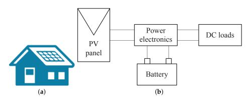
**Figure 9.** Symbolic and block diagram representations of an SHS. (**a**) Symbolic representation of a household with installed SHS. (**b**) Block diagram of an SHS.
