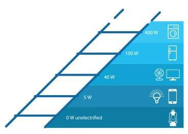
**Figure 1.** Conceptual illustration of the electrification ladder. As a household scales up the ladder, the electricity demand increases through the addition of higher power (or greater number of) appliances relative to the preceding rungs of the ladder. The power levels of the appliances are indicative only.
