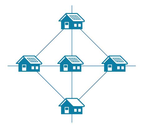
**Figure 13.** Conceptual illustration of a bottom-up, scalable, interconnected SHS-based meshed DC microgrid [32]. The bottom house is shown without any SHS, indicating the possibility of purely consumptive houses joining such a microgrid.
