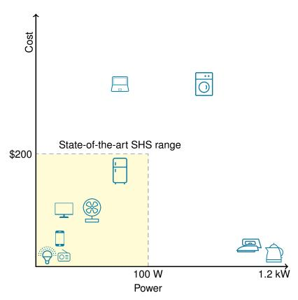
**Figure 10.** A concept graph illustrating the mapping between power rating of the various home appliances and their costs. Note: the price level is just an indicative number, as the prices differ greatly across vendors and geographies.
