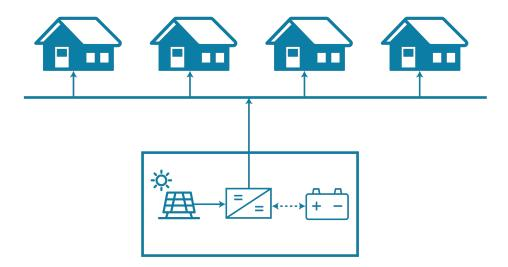
**Figure 5.** An illustration of a centralized (DC) microgrid architecture. The term centralized refers to the central power generation (solar PV) and storage (battery). Each house is assumed to have a set of (DC) loads.
