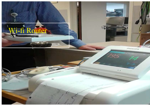
Fig. 1. The real-life example of EMI (CTG interference)
