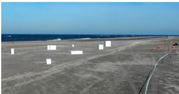
Figure 1 - Photo of one of the set-ups, with scale models of houses to test the effect of building width and height
