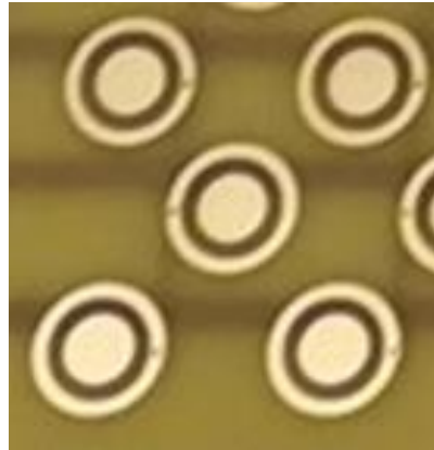
FIGURE 9. FRONT-SIDE VIEW OF A CONCENTRIC ARRAY TYPE ELECTRICAL CONDUCTIVITY SENSOR.
