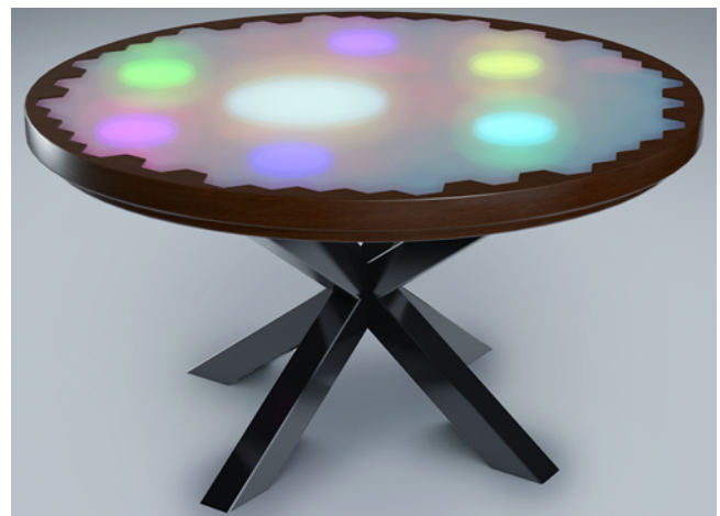
Figure 4: An illustration of the envisioned SIT, with modules for a modular setup, light interactions, and weight sensing.
