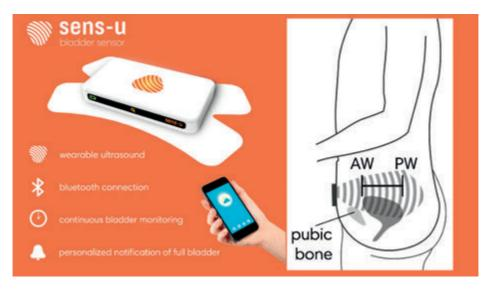
**Figure 4.1**: The SENS-U Bladder Sensor; (left) the device is positioned just above the pubic bone to monitor the axial position of the anterior (AW) and posterior (PW) bladder wall to notify the user of a full bladder (right).
