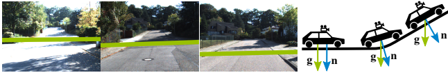
Fig. 2: Cropped images from a KITTI sequence with annotated horizon lines (left), and a sketch of the trajectory of the car with gravity vector \mathbf{g} and plane normal \mathbf{n} (right).
