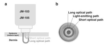
Fig. 1 Design of the evaluated TcB meters (JM-103 and JM-105). a Schematic overview of the working principle of the evaluated TcB meters. Both types of meters have the same optical design. **b** Photograph of the tip of the evaluated TcB meter with light being emitted from the illumination ring (pink). The detection rings for the long and short optical path appear as dark gray in the photograph.
