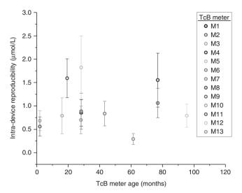
**Fig. 3 Influence of TcB meter age.** Intra-device reproducibility (average SD over all measurements and phantoms per TcB meter) as a function of time since installation in the clinic (i.e., TcB meter age). The correlation coefficient between both parameters is R=0.03. Error bars represent the standard deviation of the average SD across phantoms.
