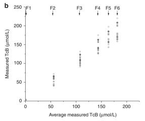
**Fig. 2 Inter-device reproducibility of TcB meters.** Measured TcB values per TcB meter (M1–M13, Table 1) and phantom (F1–F6, Table 2) as a function of **a** the absorption coefficient of the phantom at 450 nm, and **b** the average measured TcB over all meters. Error bars (standard deviation of the TcB measurements per meter) fall behind the data points.
