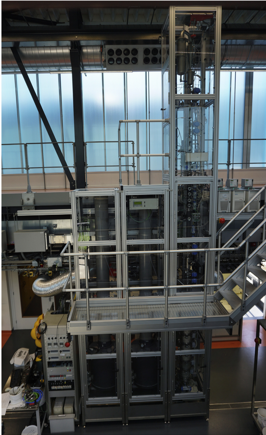
Fig. 3. Picture of the experimental pressurized MSFB setup: the right case contains the actual setup.
