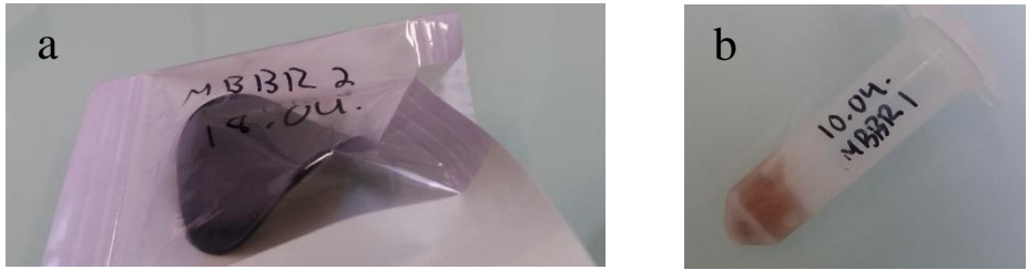
Fig. 5S. Prepared samples of the biofilm-coated carrier (a), and pellets produced from the centrifuge of the mixed liquor (b) for DNA extraction
