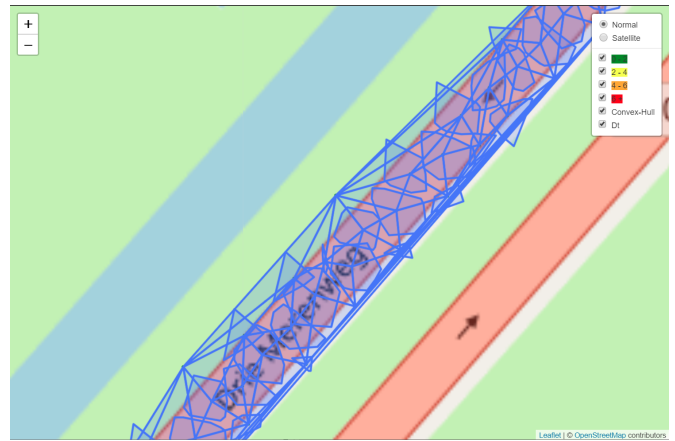
Fig. 5. Map showing a road segment with calculated DT and convex hull in street zoom level
