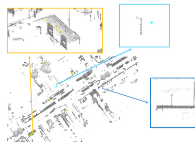
Figure 11. Several detected changes between map and MLS data in dataset 2, of which 1 (cyan box) missed the match because of having too few points in the seed.
