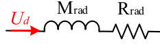
Fig. 4. The equivalent radiation impedance of the thin acoustic source using an electrical circuit in series [30].
