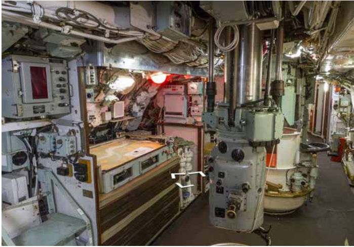
The control room of the HMS Ocelot, with the ARL table and chart table combined shown on the left of the picture
