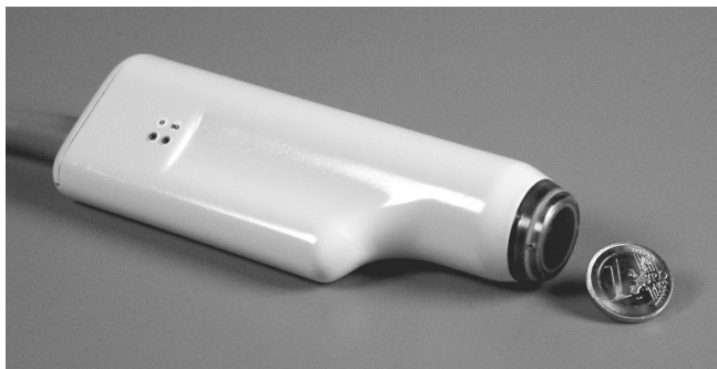
Fig. 1: Third prototype of the fast rotating ultrasound transducer.
