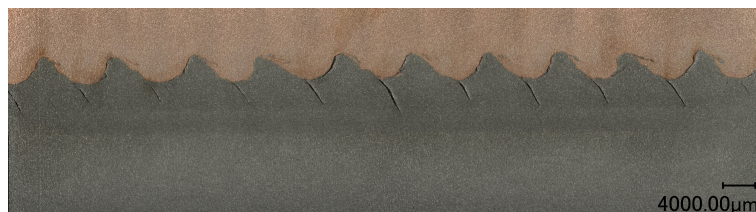
(a) Macrograph of a weld interface section in specimens of Plate 3, unetched.
