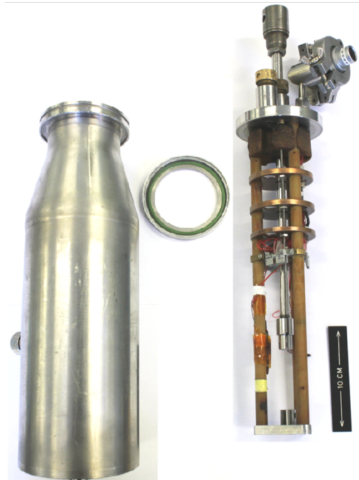
Figure 3.4: Photograph of the employed tensile cryostat as developed by CERN in the preparation of the LHC. The cryostat, with its male (right) and female (left) parts can house the sub-size specimens of figure 3.3 for cryogenic tensile testing.
