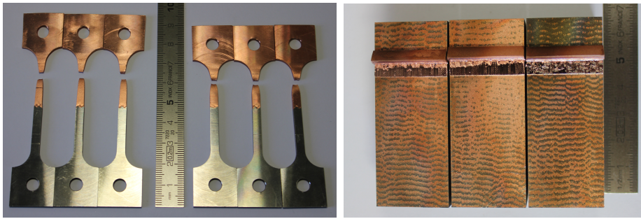
(a) Specimens of Plate 2, tested in tension, at 4.2 K (left) and RT (right). (b) Specimens of Plate 5, tested in shear, in longitudinal direction (LD).
