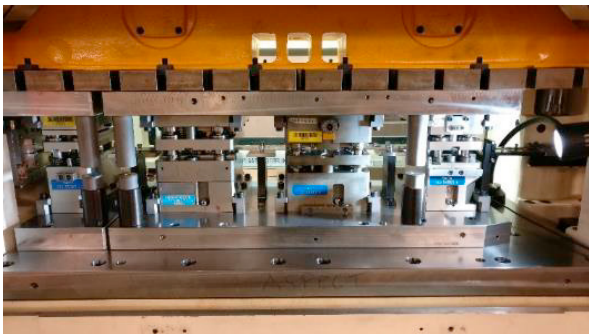
Fig. 10: Tooling for an Industrial-Scale Cold Forming Process Highly Sensitive To Temperature Induced Frictional Start-up Effects, consisting of 4 succeeding dies (named die 1 till 4 from left to right).
