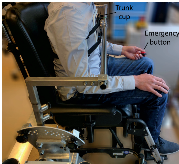
Fig. 3.2 Adult man using the Trunk Drive system at zero degree flexion angle. The trunk cup works as an adjustable connection mechanism between the Trunk Drive and the subject. The subject can operate an emergency button to stop the experiment in an unpleasant situation.
