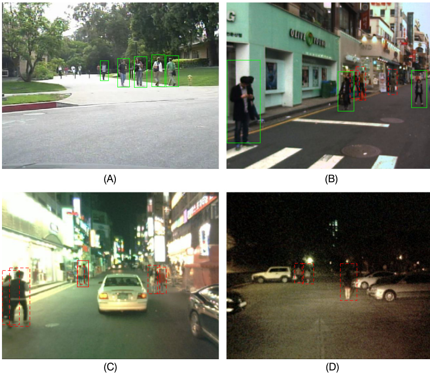
Figure 5.1 : Detections generated by a well-trained visible pedestrian detector [60]. (A) Detections generated using an image from the public Caltech testing dataset [12]; (B) detections generated using a visible image from the public KAIST testing dataset [26] captured during daytime; (C) detections generated using a visible image from the public KAIST testing dataset [26] captured during nighttime in good illumination condition; (D) detections generated using a visible image from the public KAIST testing dataset [26] captured during nighttime in bad illumination condition. Please note that green bounding boxes (BBs) represent true positives, red BBs represent false positives, and red BBs in dashed line represent false negatives.
