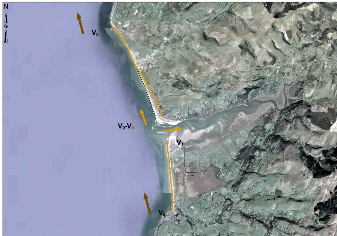
Figure 2-5: Conceptual framework for distributing a negative sediment budget (case 1). V_0 is the net longshore sediment transport capacity, V_1 (< V_0 in magnitude) is the sediment volume demand from the inlet-estuary system, the dotted black line is the initial coastline position, light brown lines indicate the final coastline position.
