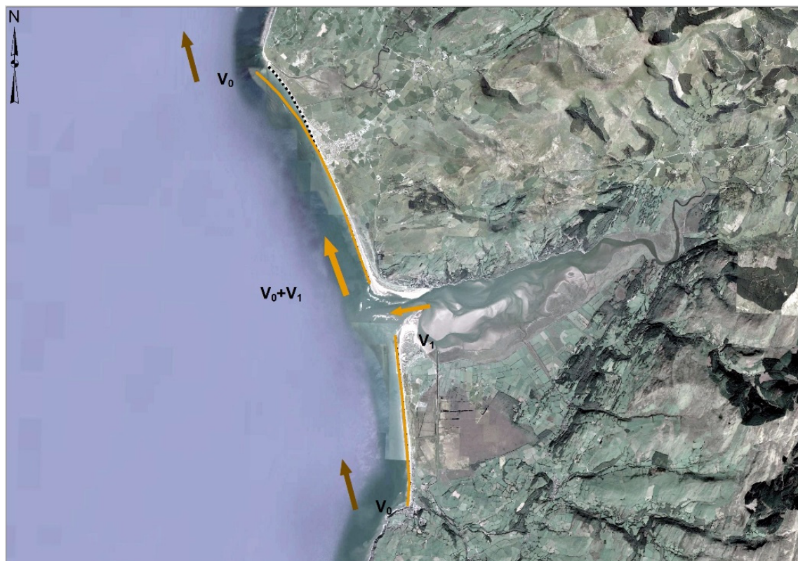
Figure 2-4: Conceptual framework for distributing a positive sediment budget. V_0 is the net longshore sediment transport capacity, V_1 is the sediment volume supplied to the coast by the inlet-estuary system, the dotted black line is the initial coastline position, light brown lines indicate the final coastline position.
