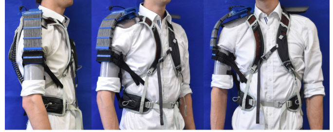
Fig. 9. Wearable proof-of-concept prototype worn by a healthy subject. This figure illustrates the actuator's potential to achieve close alignment to the body and an overall small size of the resulting assistive device.
