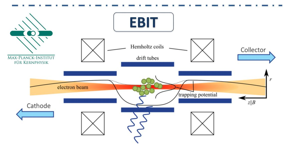
The EBIT delivers an electron beam at various, controlled electron energies
