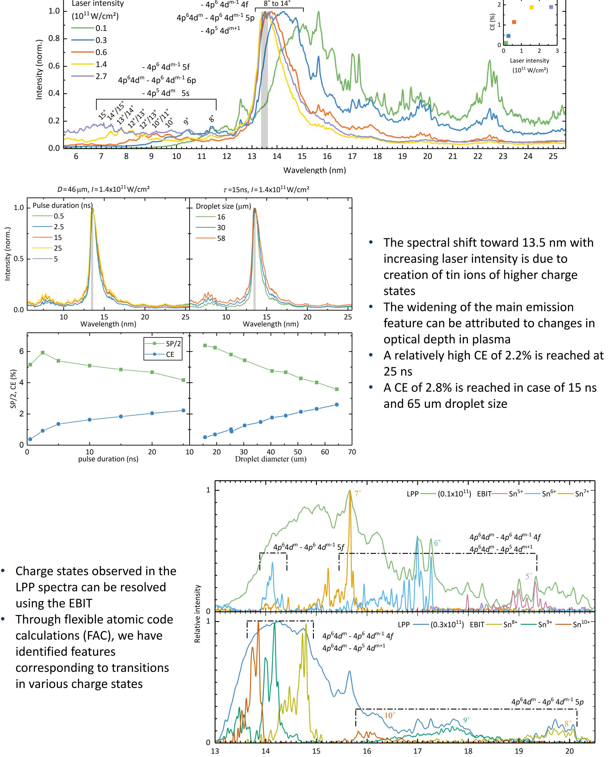
The tin droplet is irradiated by a linearly polarized, highintensity laser pulse from an Nd:YAG laser system seeded at 1064 nm
