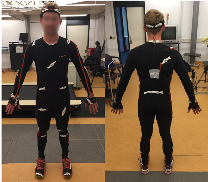
Figure 6.1: Placement of the 41 retroflective markers (according to the Plug-In Gait protocol) 1 can be seen for a representative subject. The markers were placed directly on the subject's skin. IMMU sensors were placed inside a Lycra suit, such that these remain in a fixed position with respect to the body. To accommodate the retroflective markers, holes were cut in this suit. This allowed for simultaneous measurement of kinematics using optical and IMMU motion capture technologies.
