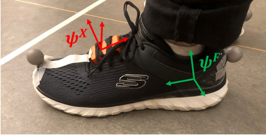
Figure 5.3: An IMU is secured under the shoelaces and its' coordinate system ( \psi^X ) is displayed in red. The retroreflective markers are places on the second metatarsal and the calcaneus, which is assumed to be a FPA of 0 degrees. The foot reference coordinate system is shown in green ( \psi^F ).
