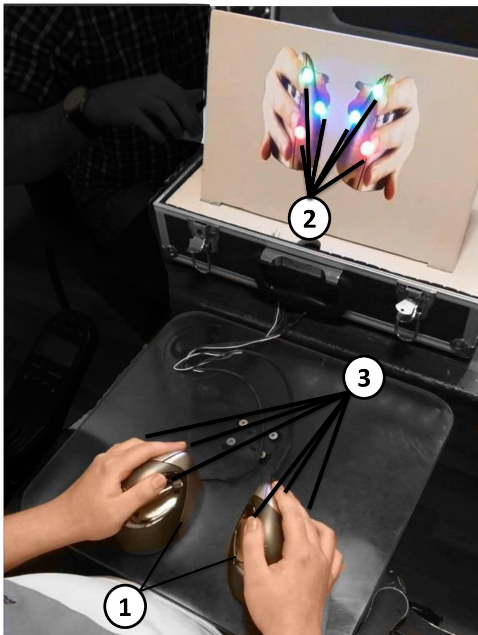
Fig 1. A participant with DMD, while using the portable setup with the proposed method, during the visuo-motor task (trial of 6 stimuli at 1 Hz). 1) Vertical mice with three buttons each. 2) LEDs: one for each index finger, middle finger, and thumb of each hand. The LEDs are also color coded: green for the index, red for the middle, and blue for the thumb; and 3) the number of fingers involved in this trial.
