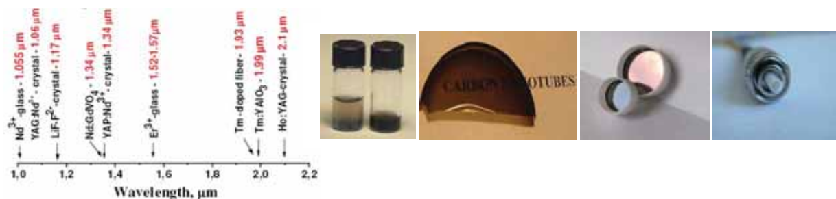
Fig. 1. a) The working spectral range of solid state lasers for whose the mode locking regime has been realized with saturable absorbers based on single-wall carbon nanotubes; b) different forms of saturable absorbers based on single-wall carbon nanotubes (from left to right: aqueous suspension, polymer composite with embedded nanotubes, coatings on mirrors, thin film on the fiber cross-section in fiber laser connector).
