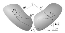
Figure 2.6: To each body a reference frame  $\psi$  is associated to express points, twists, wrenches, etc. A coordinate transformation, denoted by  $H_i^j$  changes the reference frame of expression.
