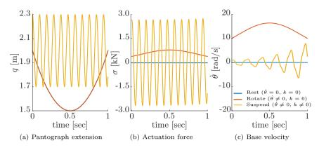
Figure 2.9: Simulation results of a dynamically balanced slider pantograph with a varying total moment of inertia, which is placed on a floating base. Three cases are simulated; with a free-floating base k=0 initially at rest  $\dot{\theta}_{\rm ini}=0$  (blue), with initial angular velocity of the base  $\dot{\theta}_{\rm ini}\neq 0$  and k=0 (red), and the base that is suspended by spring  $k\neq 0$  with an initial vibration  $\dot{\theta}_{\rm ini}\neq 0$  (yellow).
