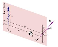
Figure 3.1: A geometrical representation of the momentum h generated by a twist t and body with a COM at c.
