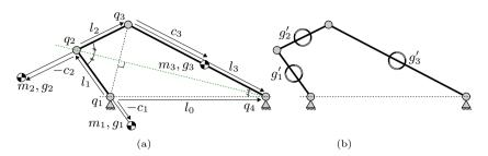
**Figure 6.3:** (a) The dynamically balanced four-bar linkage. (b) A pure-inertia dynamic equivalent of the linkage shown in (a). The green dash-dotted line shows the symmetric plane, bisecting the kite through joint  $q_2$  and  $q_4$ .
