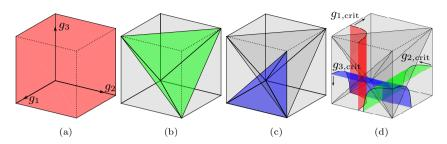
Figure 3.3: The four types of bounds on the selection of the principal moments of inertia in the balancing process. (a) positive principal moments of inertia g > 0, (b) The triangle inequality  $g_i \leq g_j + g_k$ , (c) the sorting condition  $g_1 \geq g_2 \geq g_3$  (d) and the critical principal moments of inertia (Eq. 3.32 - Eq. 3.32) for a given  $\omega$  and  $\xi_c$ .
