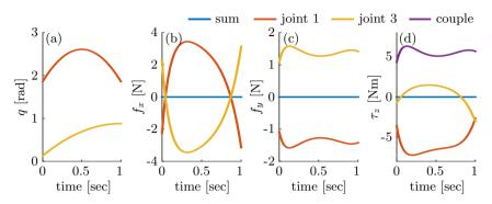
Figure 6.5: Simulation results of the novel 2-DOF manipulator. The figure shows the input angles (a), shaking forces in x and y direction (b, and c respectively) and the shaking moment (d). The shaking forces are the sum of reaction forces on the base joints (joints 1 and 3). The shaking moment is the sum of motor torques and the couple induced by base joint forces.
