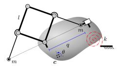
Figure 2.8: A dynamically balanced pantograph with a prismatic joint attached to a floating base. The red striped spiral denotes a torsional spring between the floating base and the inertial frame to simulate a base with a finite stiffness. Since we assume that the spring only induces a torsional stiffness, the location of attachment point has no influence and is chosen arbitrary.
