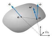
Figure 2.2: The velocity of all points  $\boldsymbol{a}$  on a rigid body are determined by the velocity  $\dot{\boldsymbol{o}}$  of a reference point  $\boldsymbol{o}$  and the angular velocity  $\boldsymbol{\omega}$ . The inertial frame is denoted by  $\psi_0$ .
