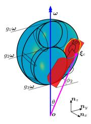
Figure 3.2: For all orientations of a body, the angular momentum  $\xi_c$  generated by angular velocity  $\omega$  will lie inside a sphere with two spherical cavities, of which the dimensions and position are determined by the bodies principal moments of inertia  $g_1$ ,  $g_2$ , and  $g_3$ . Here the orientation of the body is parameterized by  $\phi_1$ ,  $\phi_2$ , and  $\phi_3$  (currently  $\phi_3 = 0$ ) around local  $n_z$ ,  $n_x$ , and  $n_z$  axes.
