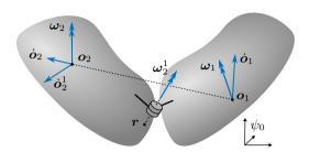
Figure 2.3: The summation of relative and absolute velocities in articulated bodies.
