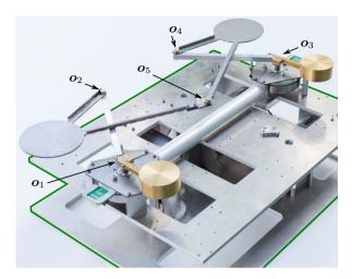
Figure 3.7: The 2-DOF dynamically balanced robot  $Fuga\ I$  mounted on a 6-DOF force/torque sensor (outlined) to measure the shaking forces and moments during motion.
