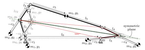
**Figure 6.4:** The dynamically balanced 2-DOF planar symmetric mechanism (a variant of the  $M_{2A}$ -type symmetric mechanism proposed in [121]). The angle bisecting pantograph-slide on the symmetry plane is shown in gray. When fixing one of the base joints the mechanism acts as a symmetric four-bar mechanism (red).
