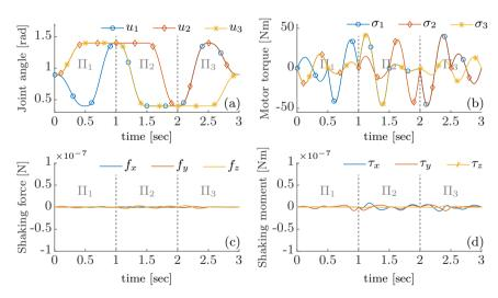
Figure 5.8: A simulation of the 3-RSR mechanism for a trajectory (a, b) over the three symmetric planes  $\Pi_i$  confirm dynamic balance as the resulting shaking forces (c) and shaking moments (d). The remaining shaking forces and moments are attributed to round-off errors in the simulations.
