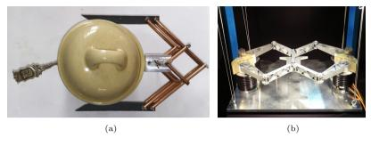
Figure 1.5: The synthesis of multi-DOF dynamically balanced principal vector linkages. (a) The mirror symmetric dynamically balanced 2-DOF gripper (from [107]). (b) The 3-DOF DUAL-V, which is dynamically balanced along its symmetry axes (from [109]).
