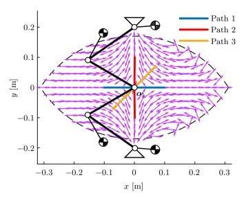
Figure 3.6: The designed mechanism permits one DOF of dynamically balanced movement, in each pose. The pink arrows indicate the corresponding traces of the endeffector  $o_5$ . Path 1 and 2 are reactionless paths that in the middle of the workspace, the instantaneous dynamic balance pose. Path 3 is the non-moment balanced path. The dashed line denotes the workspace boundary.
