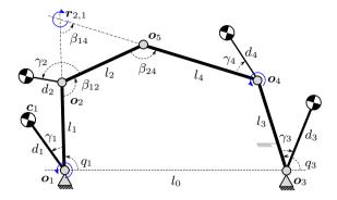
**Figure 3.4:** The kinematics of the 5R planar five-bar mechanism. The solid arrows indicate axis of rotation of moving bodies due to actuation of  $q_1$  and fixation of  $q_3$ . For body 2, the axis of rotation lies at  $r_{2,1}$ .
