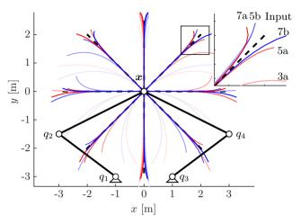
Figure 4.2: The Taylor approximation of the inverse kinematic model of a five-bar (solid grey) around evaluation point at  $\boldsymbol{x}^0 = [0,0]$  up to the 7<sup>th</sup> order for 4 different trajectories. It shows the left (a, red) and right (b, blue) estimation of end-effector trajectory (dashed black) for the order 1, 3, 5, and 7. The insert shows convergence for higher-order estimations far from the evaluation point.
