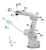
Figure 2.5: The end-effector twist  $t_{\text{see}}$  of an industrial 6-axis robot is formed by a linear combination of the instantaneous screw axis of each joint  $(s_i, \text{ for } i = [1...6])$ , passing through the shoulder  $r_s$ , elbow  $r_e$ , and wrist  $r_w$ , expressed in the inertial frame of reference  $\psi$ . (Figure adapted from Adept: Viper Six-Axis Robot (s1300 Series), accessed on 23 December 2019, www.e-motionsupply.com)
