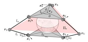
Figure 5.5: The kinematic definition of the 3-RSR. During motion the end-effector stays tangential to an expanding sphere touching the platform center and the base center [16]. This mechanism further exhibits a mirror symmetry with respect to a plane  $\Pi_s$  passing thorough the spherical joints located at  $r_2$ ,  $r_5$ , and  $r_8$ .
