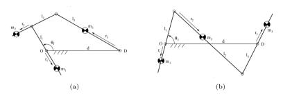
Figure 1.4: Dynamic balance of a planar 4R four-bar linkage is possible only for (a) the kite type and (b) anti-parallelogram type [75]. (Figures from [120])
