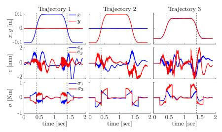
Figure 3.8: The x- and y-position of the end-effector (top row), the controller error e in end-effector coordinates (middle row) and the used motor torque  $\sigma$  (bottom row) for the three trajectories. Trajectory 1 and 2 follow the two reactionless paths through the center of the workspace. Trajectory 3 follows a non-moment balanced diagonal. The vertical lines indicate where the robot passes through the instantaneous dynamic balance pose.
