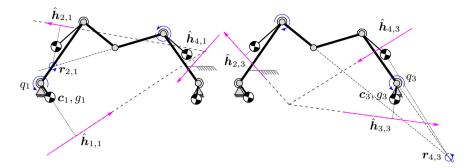
**Figure 3.5:** A graphical representation of the instantaneous dynamic balance procedure of a 5R planar five-bar. Left shows that the momentum wrenches of the bodies (straight arrows) due to the actuation of the first DOF (joint  $q_1$ ) sum to zero. Right shows the zero sum of the momentum wrenches for the second DOF, the actuation of joint  $q_3$ .
