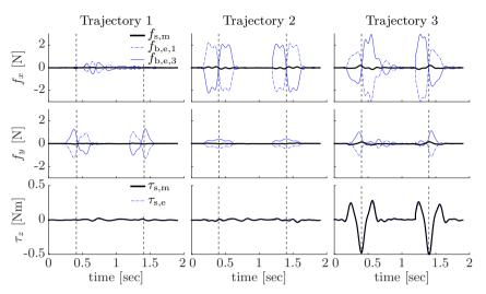
Figure 3.9: The measured shaking forces  $f_{s,m}$  (top and middle) and moments  $\tau_{s,m}$  (bottom) are shown with thick solid lines. For comparison the estimated bearing forces on the base joint are given in thin dashed and thin solid lines, respectively  $f_{b,e,1}$  and  $f_{b,e,3}$ . In the bottom row the estimated shaking moment  $\tau_{s,e}$  is shown with a thin dashed line. The vertical lines indicate where the robot passes through the instantaneous dynamic balance pose.
