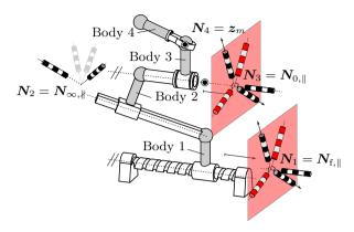
Figure 5.3: The 16 dynamically balanced design parameters of the HPRS 6-DOF serial chain. Each of the four joints permits a transfer of inertial parameters  $N_i$ .
