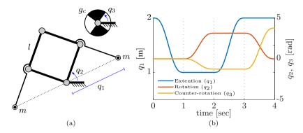
Figure 2.7: (a) A force balanced pantograph is dynamically balanced by a counterrotating inertia wheel. (b) The nonholonomic behaviour of this system can be used to reach any pose in its configuration space in a dynamically balanced manner.
