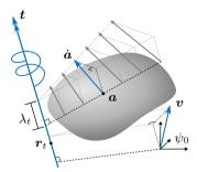
Figure 2.4: The linear and angular velocity of body form a helical velocity field for all particles a of a body. This twist t is denoted with a double arrow, with a helix representing the twist pitch  $\lambda_t$ . The velocity v is the velocity of the points instantaneously passing through the origin of reference  $\psi$ .
