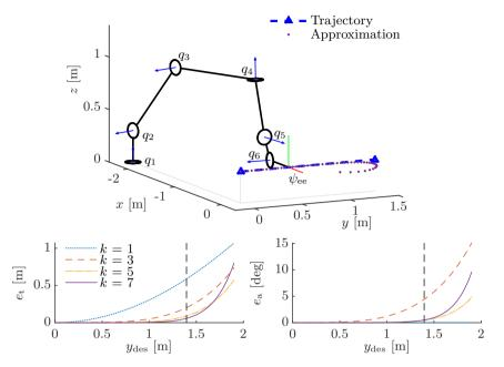
Figure 4.1: Top The 7<sup>th</sup>-order Taylor expansion of the inverse kinematic model of a 6 DOF serial manipulator (solid black) over a desired horizontal trajectory  $y_{\text{des}}$ . The evaluation point is [0,0,0.3]. The trajectory is approximated well until close to the end of the workspace at [0,1.4,0.3]. Bottom left and right The approximation error for translation  $e_{\text{t}}$  and orientation  $e_{\text{a}}$ , respectively. The vertical line denotes the end of the workspace.
