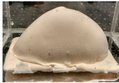
Fig. 3. Final semi-anthropomorphic photoacoustic breast phantom embedded with blood vessel mimics.
