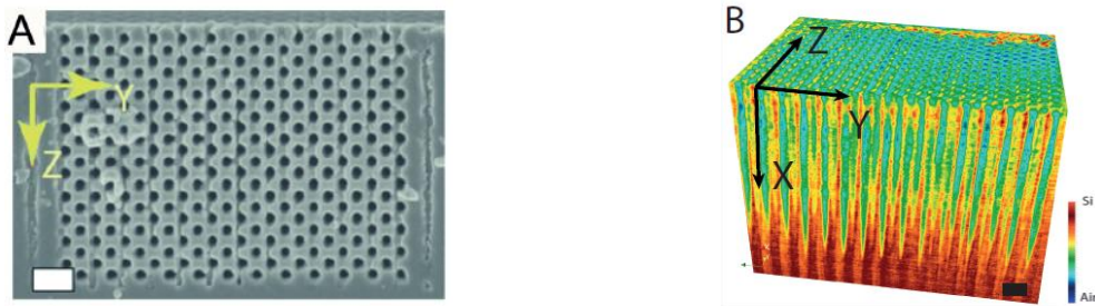
Fig. 1. (A) SEM image of the surface of a 3D Si inverse woodpile photonic crystal from Ref. [3] (B) Bird's-eye view of the sample volume of an inverse woodpile crystal reconstructed from X-ray tomography [5] with 20 nm resolution. The colour scale is the 3D material density \rho(X, Y, Z) interpolated between air and Si, the latter set to 255.
