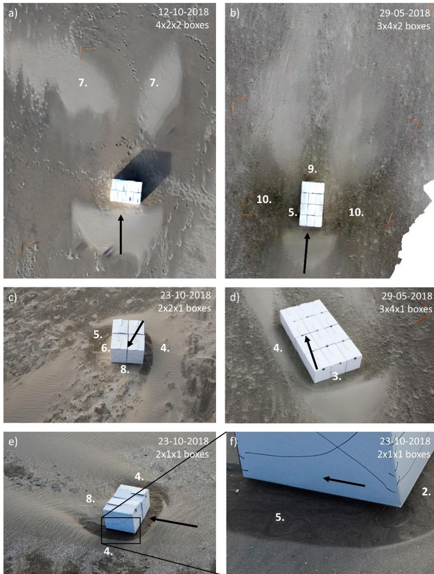
Figure 6: Notable erosion and sedimentation structures around scale models, with arrows indicating the wind direction. 6a) Orthophoto showing a large distance between the model and the start of the downwind horseshoe deposition. 6b) Orthophoto showing lateral inner and outer erosion and downwind inner erosion. 6c) Photo of a model oriented obliquely to the wind, showing lateral inner deposition 6d) Photo of model a oriented obliquely to the wind, showing upwind inner deposition and asymmetric lateral deposition. 6e) Photo showing continuous lateral deposition. 6f) Zoom of 6e, showing erosion around model and under model corners.
