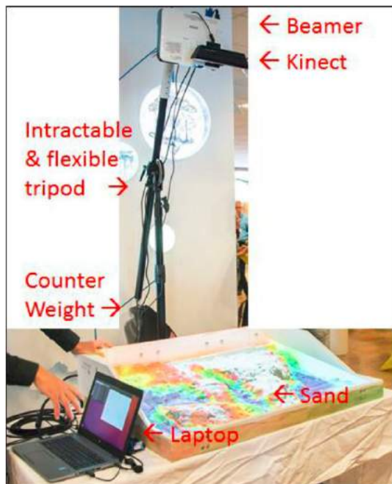
Figure 1. SandBox setup and interface (photo from Ottevanger et al., 2017)
