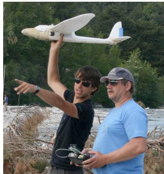
Figure 1. Fixed wing aircraft with aboard a Canon Powershot D10 RGB camera. The drone is manually controlled and flown at an elevation of ~ 130m.
