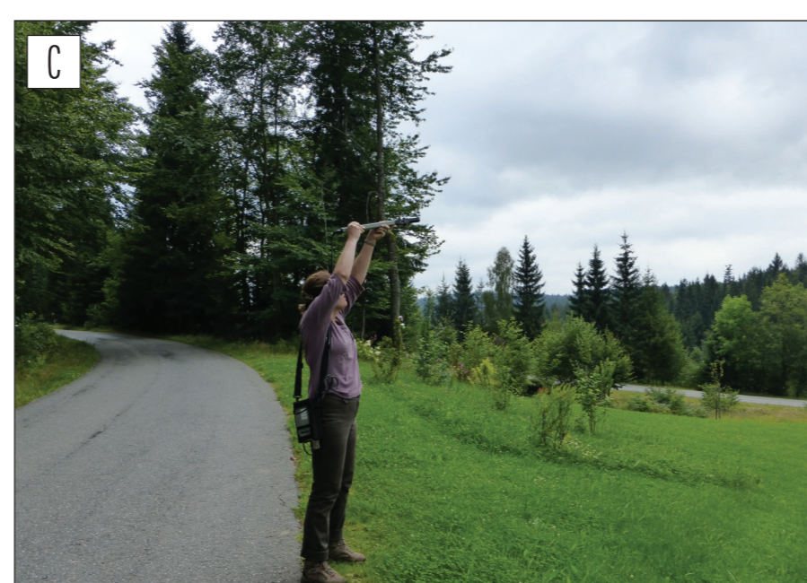
Figure 2. The field campaign was conducted in the Bavarian Forest National Park (a), digital hemispherical photographs acquired during the field campaigns in 2015 (b), and a plant canopy analyser was used to measure leaf area index (c).
