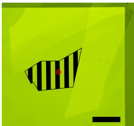
Figure A3.7: Optical image of pristine graphene placed on SiN membrane. The dark green area is that where the membrane is supported by the silicon substrate while the lighter green square is the suspended membrane. The lightest green patches are the exfoliated graphene with lighter green indicating more layers of graphene. The monolayer region is shaded with stripes and the location of the nanopore in the SiN membrane is indicated with a circle and crosshair. The flake of exfoliated graphene has been placed such that the nanopore is near the edge of the flake. Scale bar is 20 microns.
